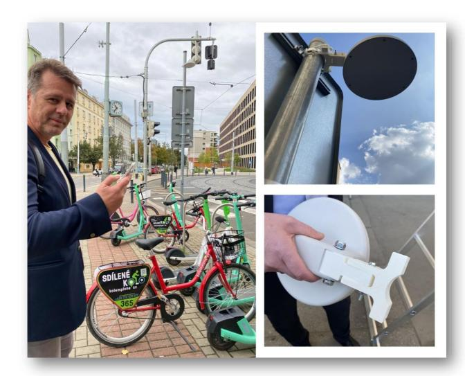
The pilot project is currently being tested in Prague 7, where suitable locations have been identified in collaboration with the Department of Transport. In these 25 pilot locations, high-precision Bluetooth sensors have been installed and the parking zones have been calibrated to ensure that shared bikes and kick-scooters respond accurately to the designated areas. The use of a shared mode of transport cannot be terminated until it is in a precisely defined parking zone.
